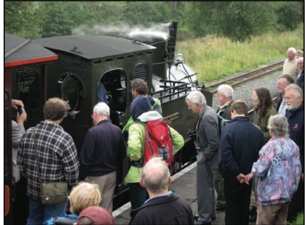
8: Watching the engine being coupled at Kirkhaugh The 90 hp 0-4-0 tank locomotive no. 125 "Thomas Edmondson" was built in 1918 to a standard First World War German Army design by Henschel & Sohn of Kassel, Germany.
