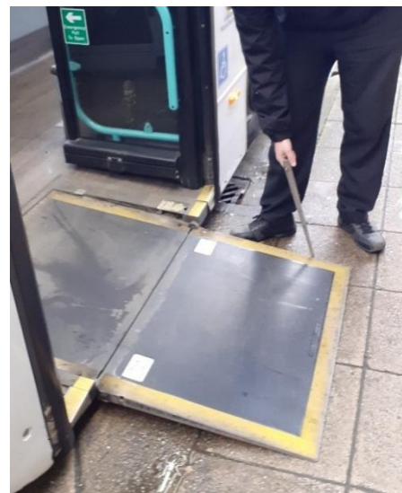
Showing the operation of the wheelchair bridge on DalesBus 874
